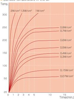
The heater itself is measured in the air at room temperature. The surface temperature of the heater changes depending on the operating environment, the material of the heating object, shapes, etc.
