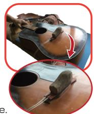
The best heater for removing the bridge.
