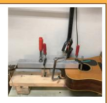
Can be used to fix curving area of the neck.
